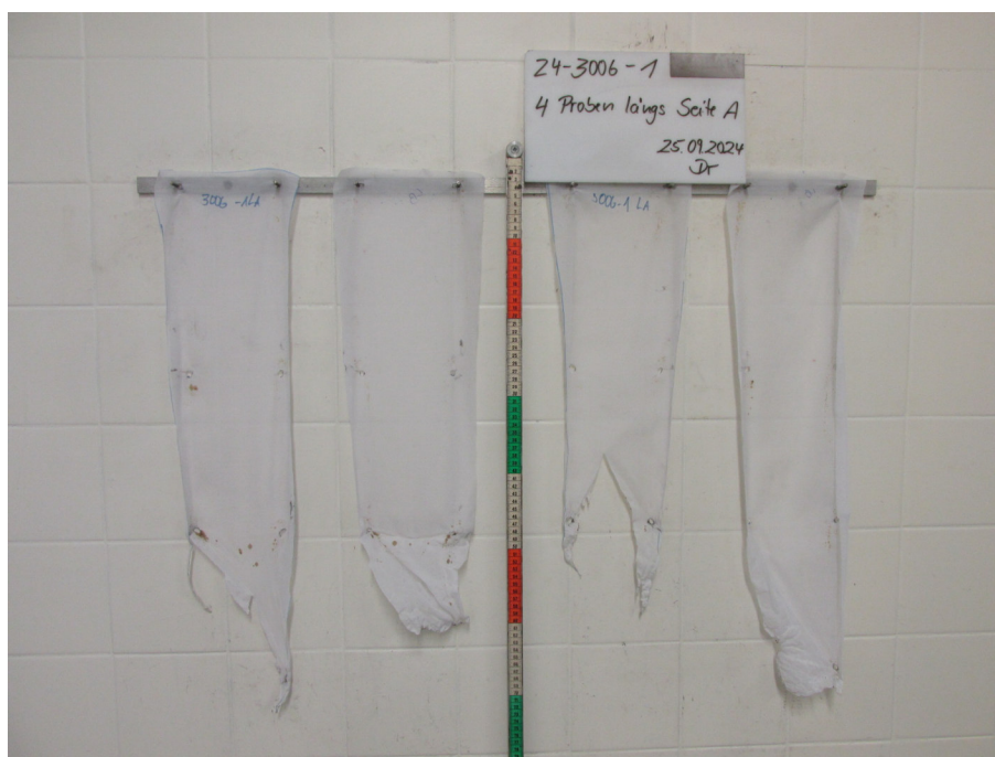
fig 2: Photo of test specimen after the test
