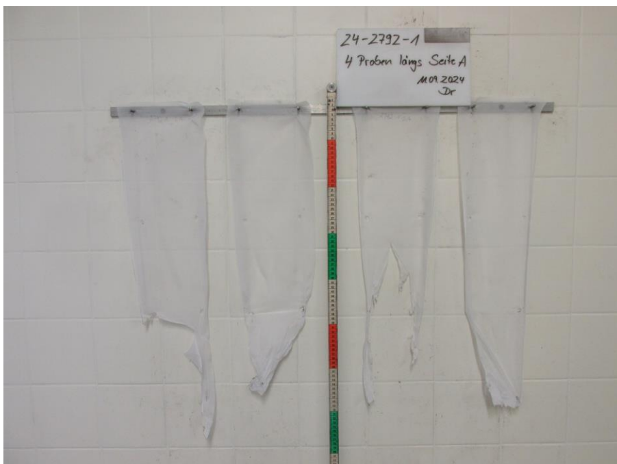
fig 2: Photo of test specimen after the test
