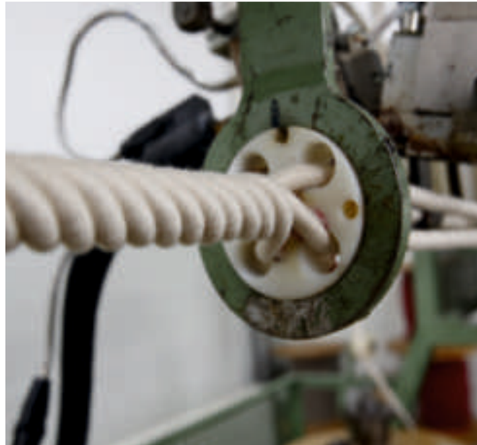
Detail of a 7 meters long Gerster Stair Rope Machine
